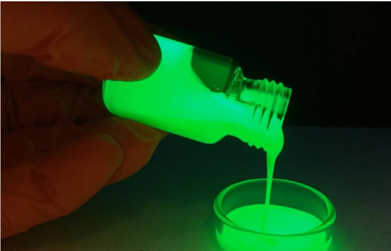
that convert X-rays into visible light. BrightSplash™, its second product, is a resin formulation that allows third parties to use their own PQD-containing devices and polymer film for photon conversion. BrightSplash™ is of particular interest to manufacturers of displays as it permits production of the latest generation of LCDs with the purest and most vivid colours.
