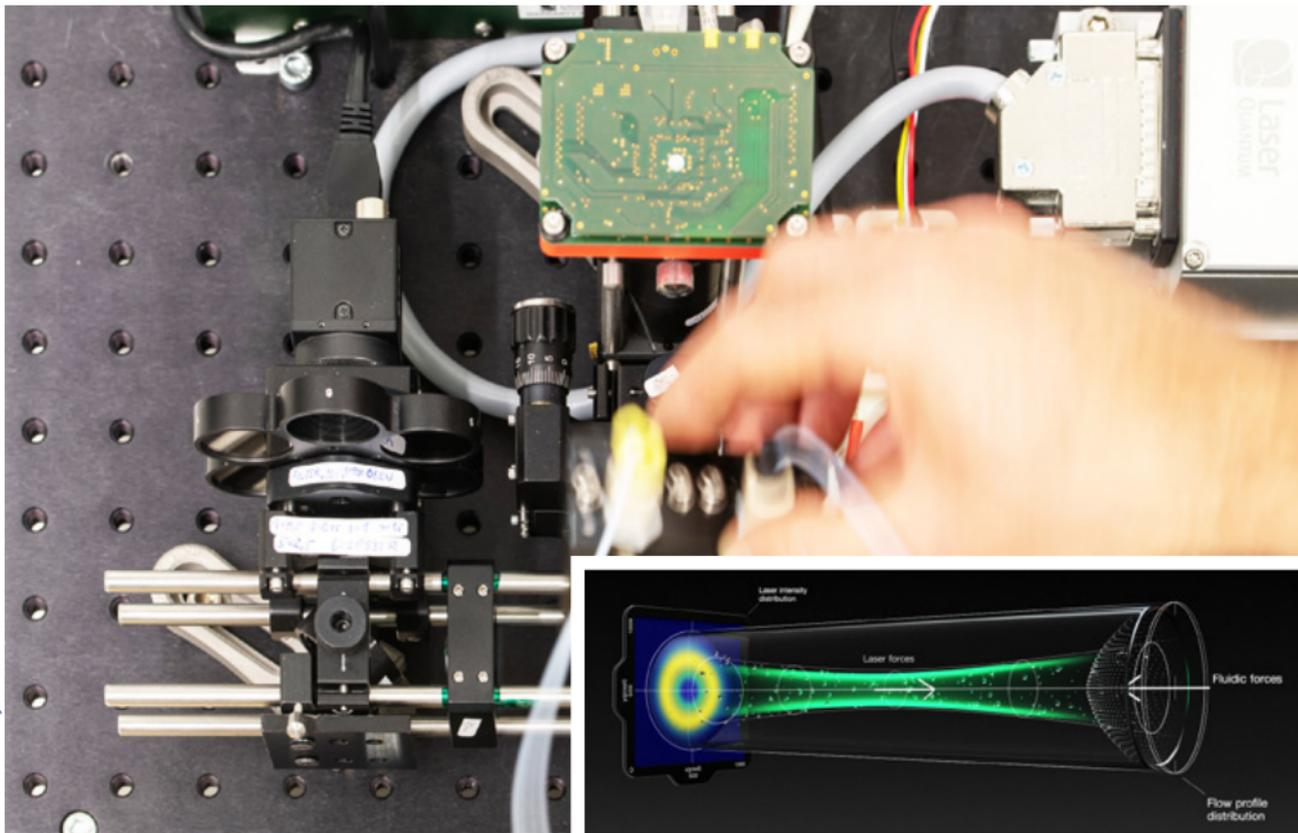
nanoparticles can be continuously and automatically characterised in real time. Sophisticated evaluation algorithms make it possible, for the first time, to collect statistically relevant characterisation data of the particles responsible for the quality of the product during the manufacturing process.
